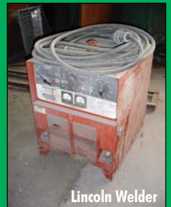
Lincoln Model Idealarc R3S-325 Arc Welder
